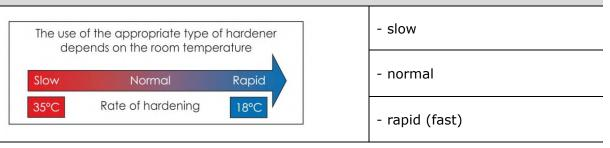
The type of used hardener affects coating drying time and depends on room temperature and the preference of the painter. Proper selection of the type of hardener ensures appropriate structure and appearance of coating.
